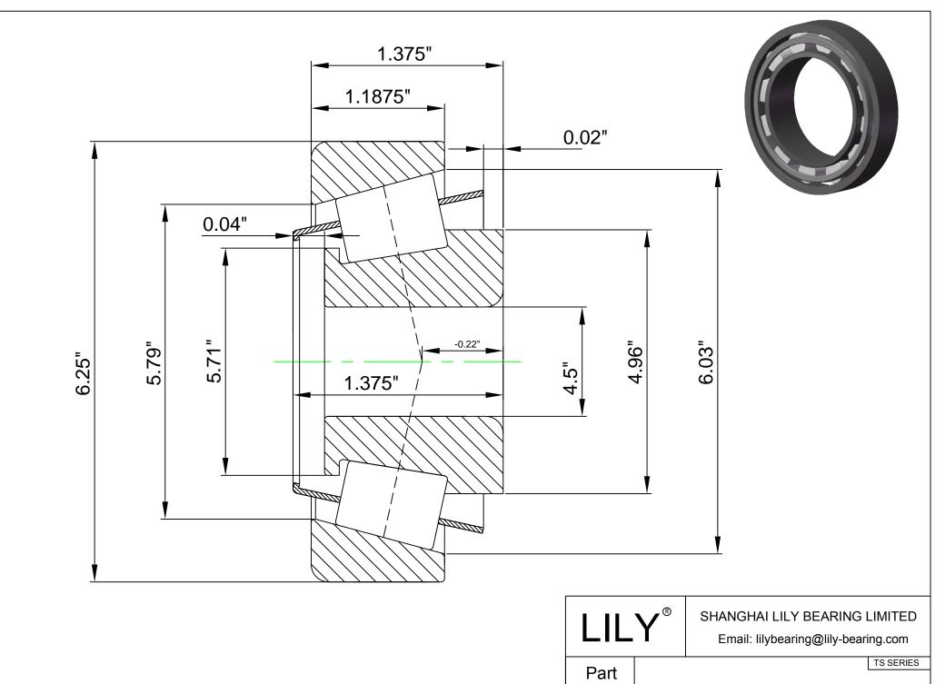
LM122948-LM122911(Tapered Single Roller Bearings)
