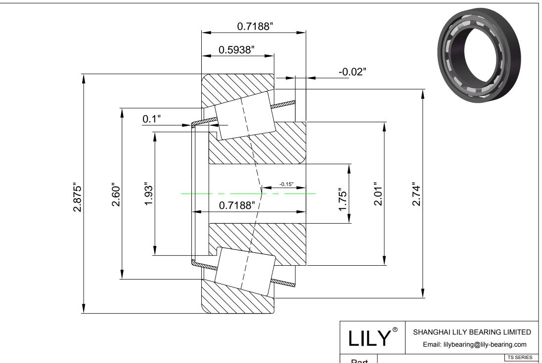
Part L102849-L102810(Tapered Single Roller Bearings) Number
