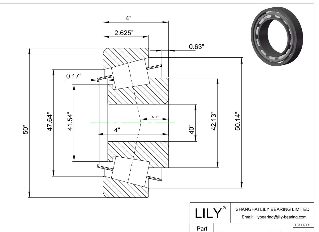
EE168400-168500(Tapered Single Roller Bearings)
