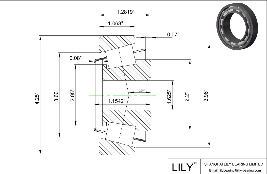
TS SERIES Part 464-452A(Tapered Single Roller Bearings) Number
