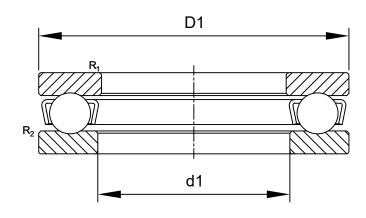
R<sub>1,2</sub>: min0.15 mm Chamfer Dimension Washer
