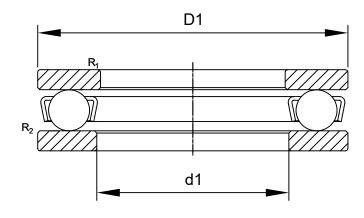
R<sub>1,2</sub>: min0.15 mm Chamfer Dimension Washer
