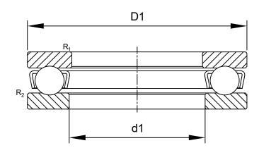
R<sub>1/2</sub>: min0.6 mm Chamfer Dimension Washer
